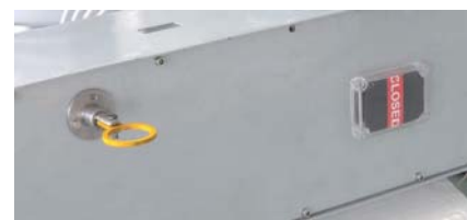
Lockout handle-push in (close position)
