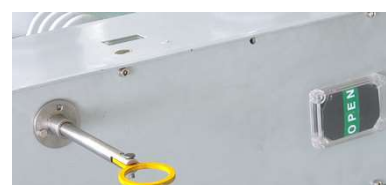
Lockout handle-pulled (open position)
